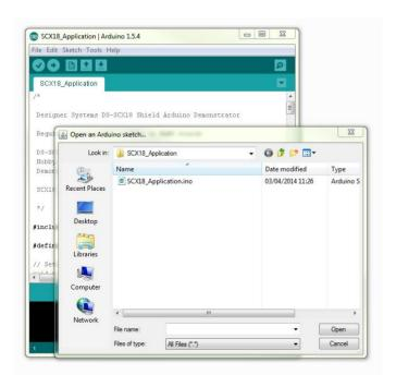
Connect the Arduino board to the computer using a USB cable and power up the board with an external power adaptor. Within the Arduino environment click on 'File' then 'Upload'. (Note: This assumes that you have already selected the Arduino board and COM port using 'Tools', 'Board' or 'Port')
